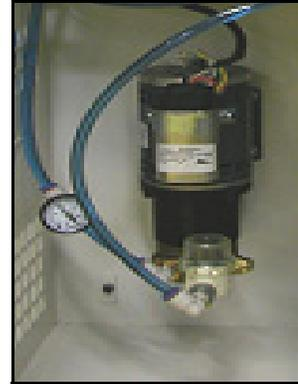
Figure 1-7: Pump Filter
