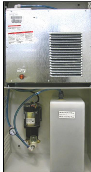
Figure 1-6: Spindle Cooling System
