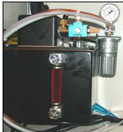
Figure 1-2: Way Lube Oil Reservoir
